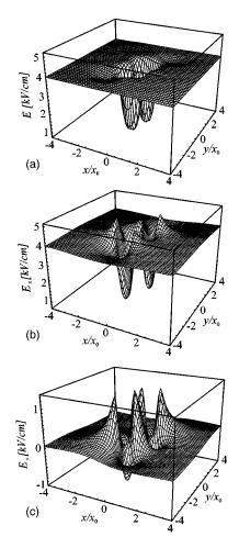
FIG. 3. Surface plots of the components of the space-charge field from Fig. 2 at z = 11.3 mm. (a)  $E_x$  of the isotropic model; and (b)  $E_x$  and (c)  $E_y$  of the anisotropic model.
