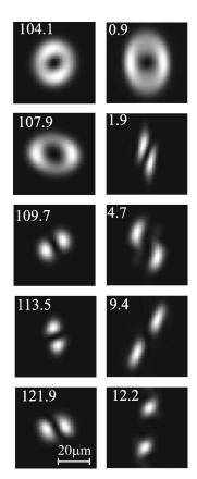
FIG. 4. Breakup during propagation of the vortex component of a vector soliton. Left column, the isotropic model; right column, the anisotropic model. Even though the breakup phases appear similar, note the widely different propagation distances in each of the figures. Initial intensities of the fundamental (not shown) and of the vortex component were  $I_0=9$ , and other parameters are as in Fig. 1.
