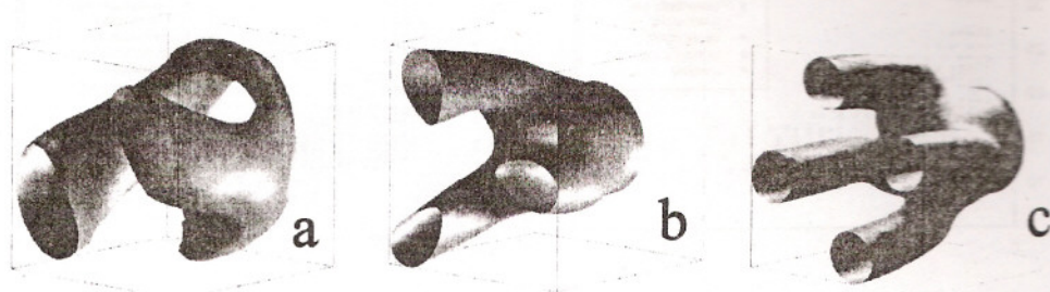
Fig. 8. Standing waves. Isosurface plots of (a) stable dipole, (b) stable tripole and (c) stable quadrupole. The corresponding parameters are as in Fig. 7 (a), (b) and (d), respectively. The isosurfaces at half-maximum intensity are plotted in the direct space, with the transverse plane being vertical and the z axis horizontal.
