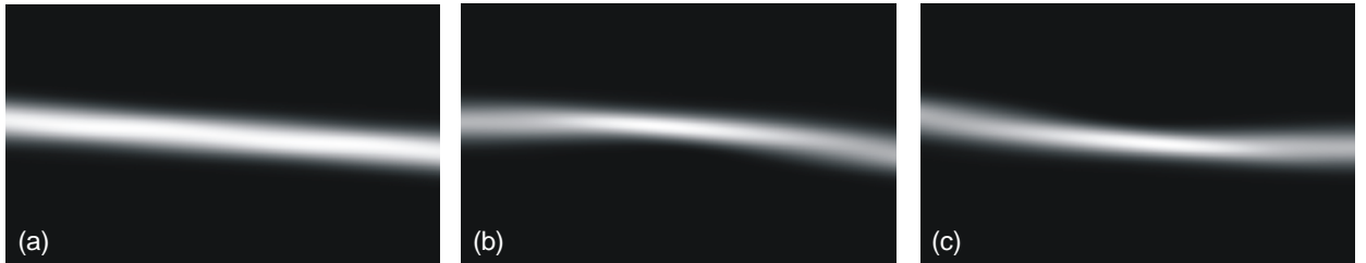
Fig. 9: Counterpropagating self-trapped waveguide formed out of two coherent beams. a) Resulting spatial intensity distribution in steady state, b) right-propagating beam, c) left-propagating beam. The size of the data windows is 10 beam diameters in the transverse direction and two diffraction lengths in the direction of beam propagation. The initial integrated intensities are |F|^2 = |B|^2 = 1 , the coupling strength is \Gamma = 5 .
